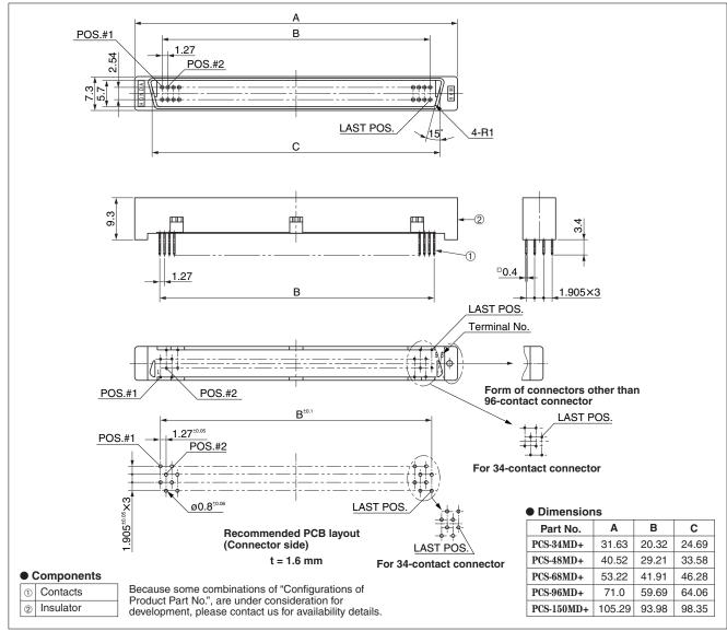
Mating connectors: PCS series PCB-side through hole type female connector
